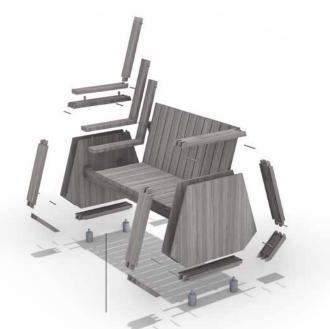
The single-component design with material-pure (metal-free) connection points as a plug-in system guarantees complete detachability and recyclability without residues and sorted by type.
